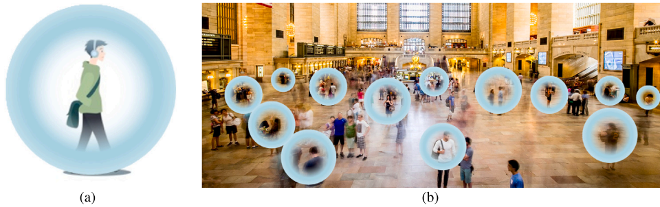
Fig. 1. (a) A magnetic bubble around an user's PAN. (b) This small bubbles ensure a significant amount of spatial reuse of the same frequency in a crowded area.
