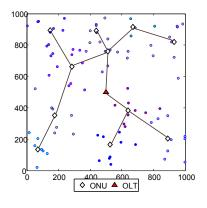
Fig. 13. Fiber layout using minimum spanning tree for uniform distribution of mesh routers.
