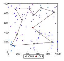
Fig. 16. Fiber layout by solving the travelling salesman problem for uniform distribution of mesh routers.
