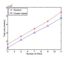
Fig. 10. Comparison of overall cost for random placement and clustering-based schemes for non-uniform distribution of mesh routers.
