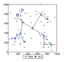
Fig. 14. Fiber layout using minimum spanning tree for non-uniform distribution of mesh routers.
