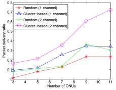
Fig. 6. Comparison of delivery ratio with different number of ONUs for random placement and clustering-based schemes for uniform distribution of mesh routers.
