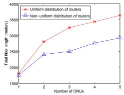
Fig. 18. Comparison of total fiber length required for ring PON architecture for uniform and non-uniform distribution of mesh routers.
