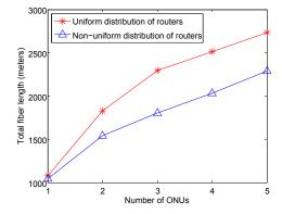
Fig. 15. Comparison of total fiber length required for tree PON architecture for uniform and non-uniform distribution of mesh routers.
