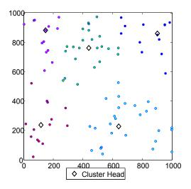
Fig. 2. The placement of ONUs in a random distribution of mesh routers.
