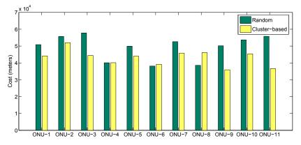
Fig. 9. Costs of different ONUs for random placement and clustering-based schemes where mesh routers are non-uniformly distributed.
