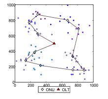
Fig. 17. Fiber layout by solving the travelling salesman problem for non-uniform distribution of mesh routers.
