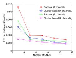
Fig. 7. Comparison of end-to-end delay with different number of ONUs for random placement and clustering-based schemes for uniform distribution of mesh routers.
