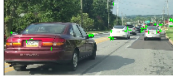
Fig. 2: Keypoint based characterization of a frame (ORB).
