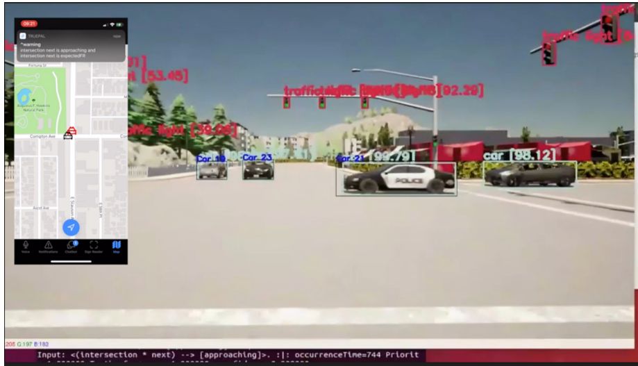
Fig. 3: Scenario 1.3.1: TruePAL warns that the user is approaching the next intersection at the same time as another first responder / TruePAL vehicle. The warning is given far enough in advance that the first responder can brake and prevent the collision.
